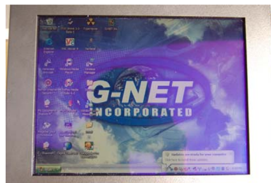
The photo above shows the display in direct sunlight, when equipped with the transflective panel option.
